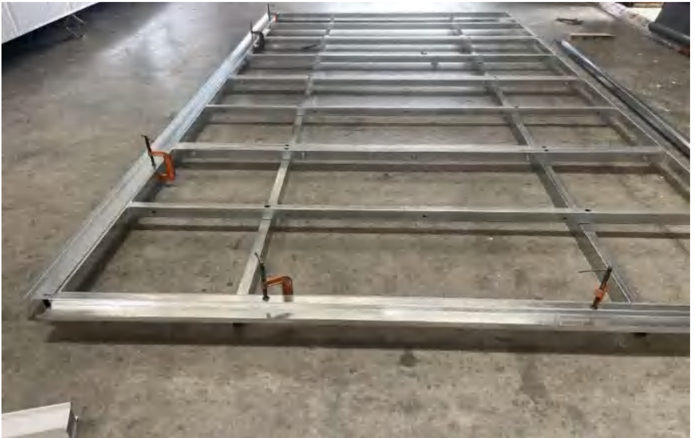
Use the clamps to secure the U channel to the chassis.
